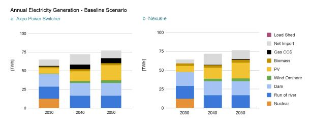
Figure 5: Annual Electricity Generation in Baseline Scenario in a. Power Switcher and b. Nexus-e
