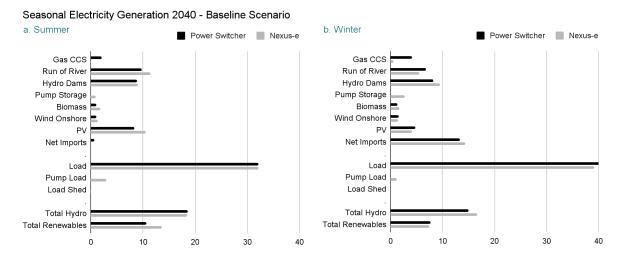
**Figure 8:** Comparison of seasonal electricity generation in 2040 in the Baseline Scenario in **a.** summer and **b.** Winter. The value for load presented here does not include efficiency losses for pumps and batteries.
