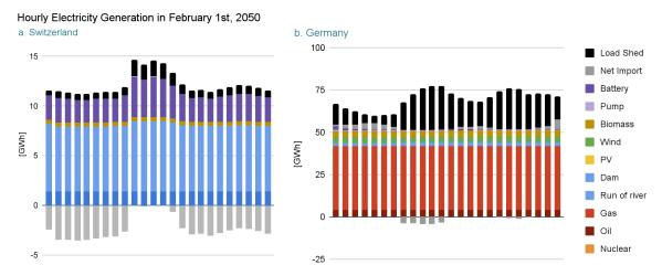
**Figure 14**: Hourly electricity generation on February 1st in 2050 for the Deficit Generation and Demand scenario in **a**. Switzerland and **b**. Germany.
